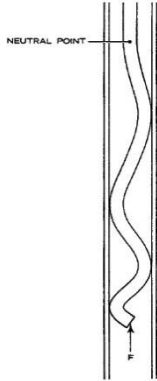
Figure 1 Tubing string bends and coils helically
