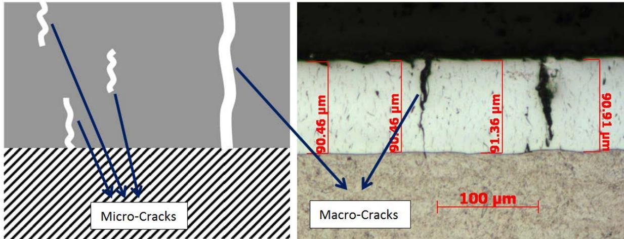
Figure 1. Micro and macro-cracks in Chrome plating.
