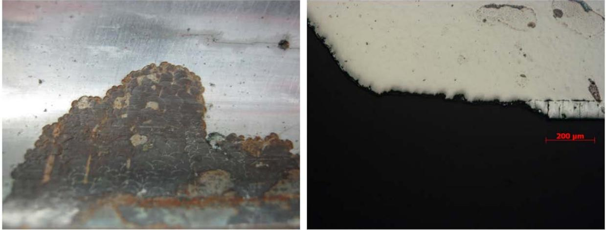
Figure 6. Flaked Chrome coating on the barrel surface.
