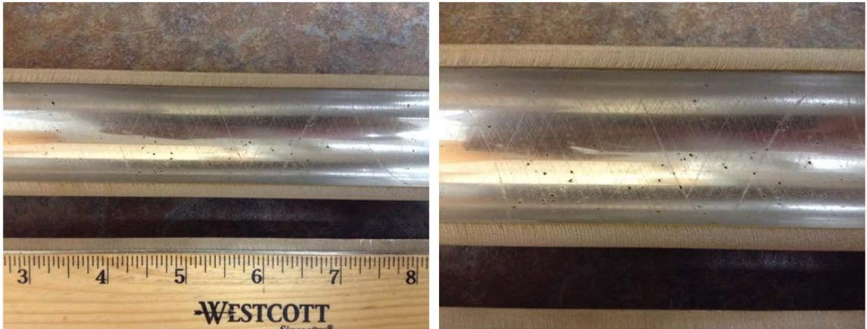
Figure 4. Helical honing marks on the barrel surface.
